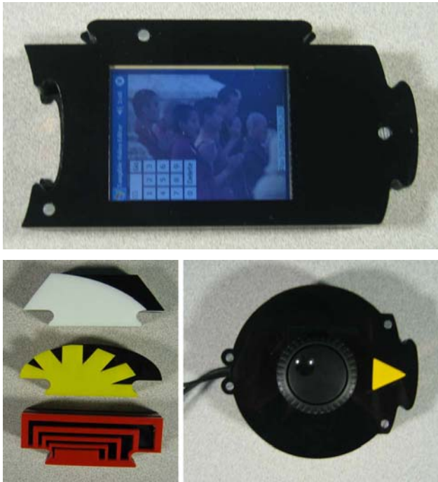
Figure 4. Counterclockwise from top: clip-holder, transitions (fade, rotate, minimize), and the play-controller.
