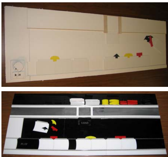
Figure 2. Foam core and plastic prototypes.
